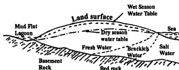
Fig. 5. Schematic cross section of Nilaveli coastal aquifer
