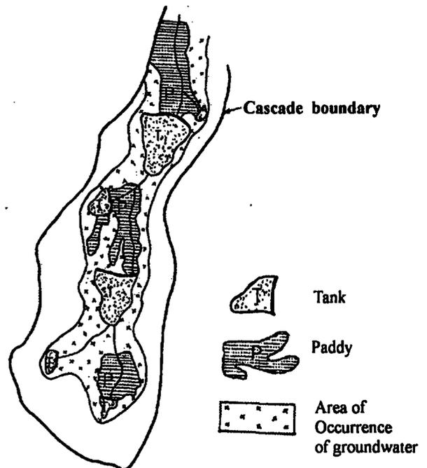
Figure 3. Schematic Representation of Groundwater area within a Cascade
