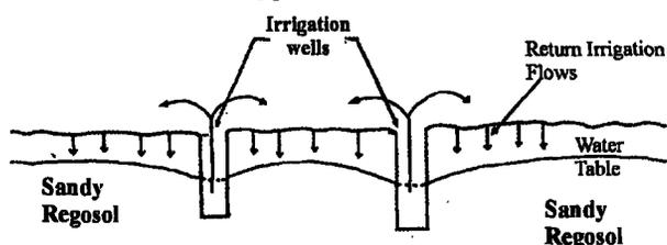
Fig. 6. Groundwater flow dominated by abstraction from Irrigation wells
